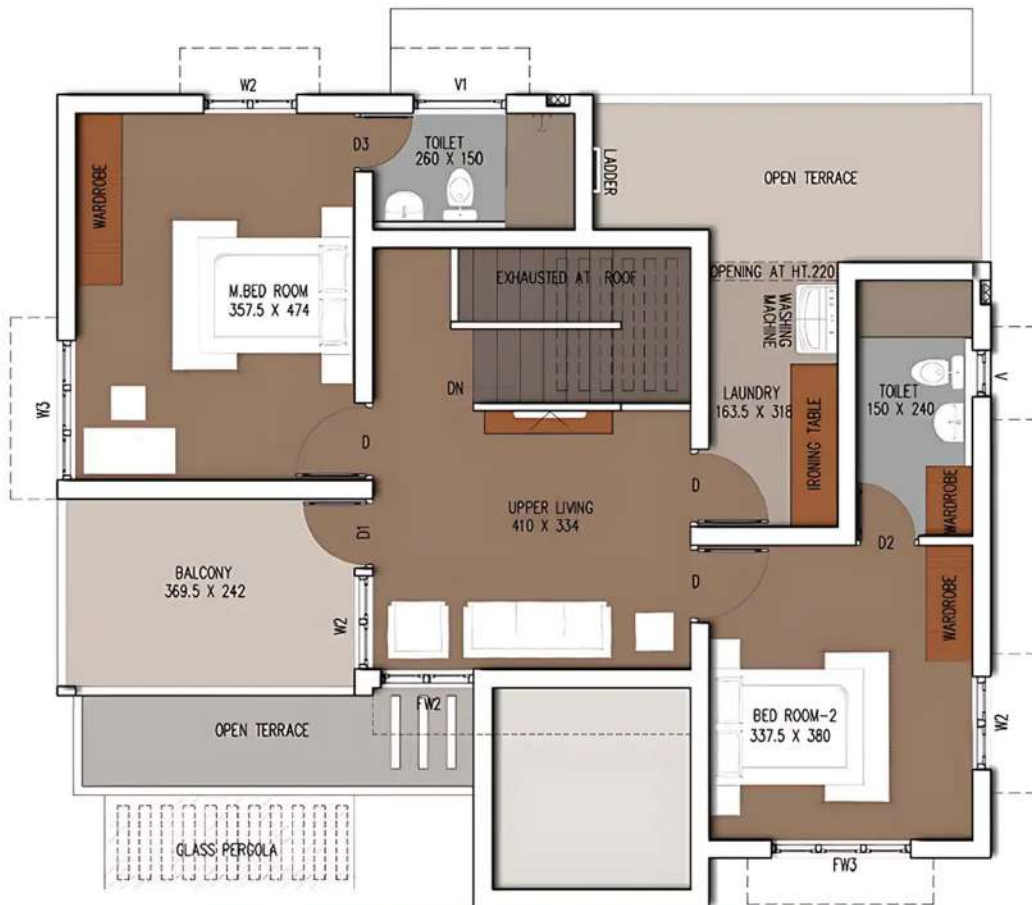
TYPE A - FIRST FLOOR - 937.41 SQ.FT. (TOTAL AREA - 2183.09 SQ.FT) FURNITURE, FITTINGS, APPLIANCES ETC SHOWN HERE ARE FOR VISUALIZATION PURPOSE ONLY
