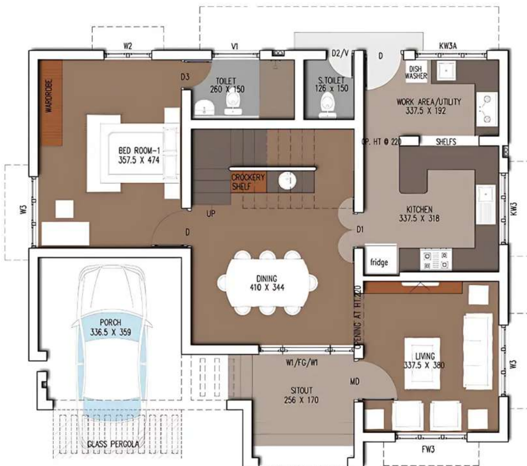
TYPE A - GROUND FLOOR - 1245.68 SQ.FT (TOTAL AREA - 2183.09 SQ.FT) FURNITURE, FITTINGS, APPLIANCES ETC SHOWN HERE ARE FOR VISUALIZATION PURPOSE ONLY
